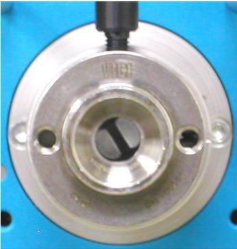
Once the rotor has been extracted, you will be able to see inside the valve to the actuator. (left)
