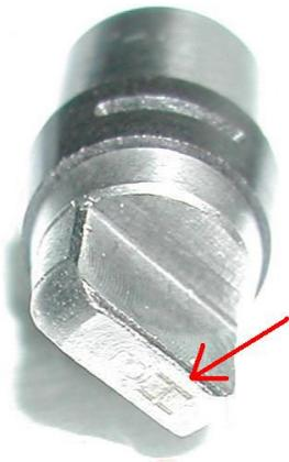
Once the rotor has been cleaned or replaced, begin by examining the back of the rotor. A small H appears on one side of the lip. This letter indicates that the material is Valcon H, a Teflon polymer. When inserting the rotor back into the valve head, this H must be oriented so the H is on the bottom half of the valve. If inserted upside-down, the valve will not work correctly.
